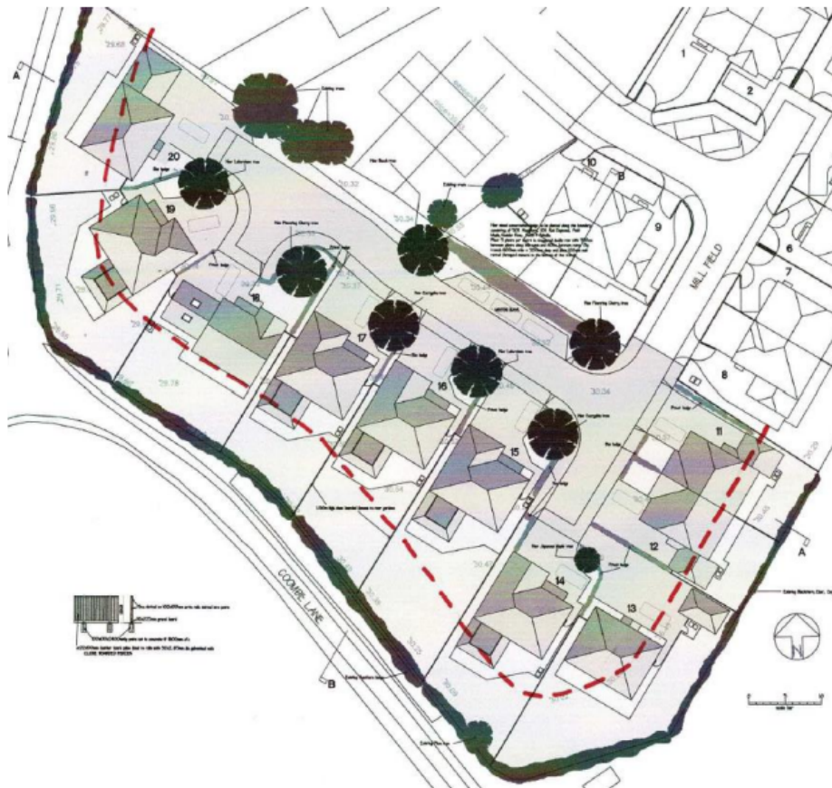
Extract from the proposed site plan 2021-09-01. The dotted red line shows the approximate extent of a 10m buffer zone of boundary screening as required by NDP Policy ANP7c
